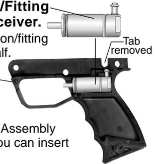
**Step 5: Prepare Upper Receiver for Response Trigger Parts Installation**
