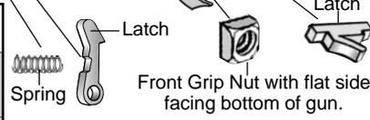
4) Use your finger tips to guide the left half straight down on to right half until receiver halves fit flush. If it does not fit flush the first time, check to make sure the spring and other parts have stayed in place and repeat until halves fit flush.
