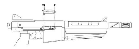
2. Inspect the leaf spring. It should be straight with a triangle at one end.
