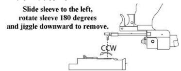
c. Remove the hammer, hammer spring and bolt from the sleeve. If they are still connected, press on the end of the sear while firmly holding onto the hammer and bolt.
