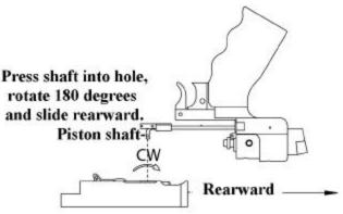
j. Align piston coupling with slot in receiver, then insert rear housing and sleeve. Install rear top screw first, followed by the other top and side screws. Caution: Do not over-tighten top or side screws.
