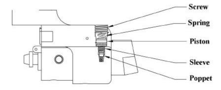
h. For reference, another view of the regulator system with parts enlarged is shown below:
