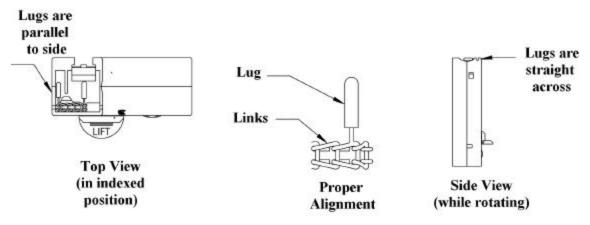
b. Binding is the result of a mis-aligned lug or link. To realign a lug, hold the chain firmly against the top roll plate with thumb and realign lug with a finger. View all sixteen lugs to make sure they are parallel to the side of the magazine and straight across the top, as shown above.
