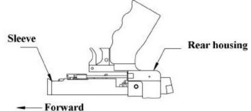
b. Slide sleeve forward, or to the left, until it clears the groove in rear housing. Rotate 180 degrees counter-clockwise. The sleeve should easily come off of the piston shaft by gently jiggling the sleeve.
