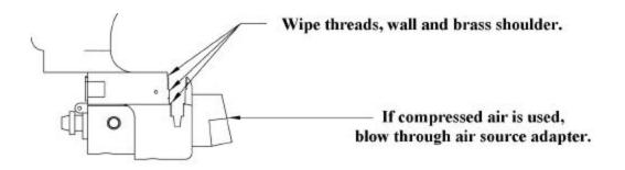
f. Before re-assembling, make sure that all regulator components are clean and free of fibers.
